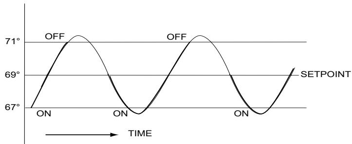
The ON-OFF controller is used in some industrial control applications, but is not practical in the majority of industrial control processes.
