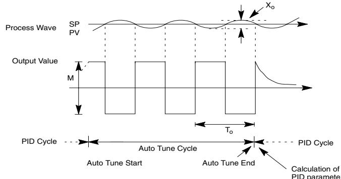
\* $M_{max}$  = Output Value upper limit setting.  $M_{min}$  = Output Value lower limit setting.
