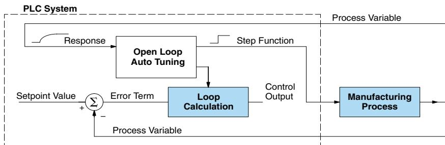
**NOTE:** In theory, the SP value does not matter in this case, because the loop is not closed. However, the requirement of the firmware is that the SP value must be more than 5% of the PV range from the actual PV before starting the auto tune cycle (for the DL205, 12 bit PV should be 205 counts or more below the SP for forward-acting loops, or 205 counts or more above the SP for reverse-acting loops).
