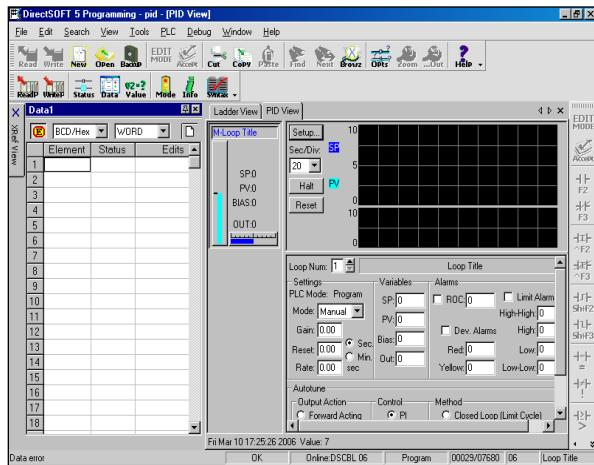
With both windows positioned in this manner, you are able to see where the PID values have been set and see the process that it is controlling. In the diagram below, you can see the current SP, PV and Output values, along with the other PID addresses. Refer to the Loop Table Word Definitions (page 8-20) for details on each word in the table. This is also a good data type reference for each word in the table.
