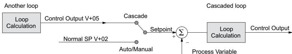
As pictured below, a loop can be changed from one mode to another, but cannot go from Manual Mode directly to Cascade, or vice versa. This mode change is prohibited because a loop would be changing two data sources at the same time and could cause a loss of control.
