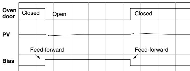
The step changes in the bias are the result of our two feed-forward writes to the bias term. We can see the PV variations are greatly reduced. The same technique may be applied for changes in setpoint.
