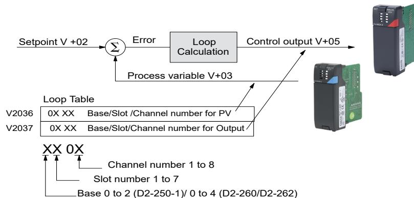
When these loop table parameters are programmed directly, a value of 0102 in register V2036 directs the loop controller to read the PV data from channel 2 of the analog input module in slot 1. A value of 0000 in either register tells the loop controller not to access the corresponding analog value directly. In that case, ladder logic must be used to transfer the value between the analog input and the loop table.
