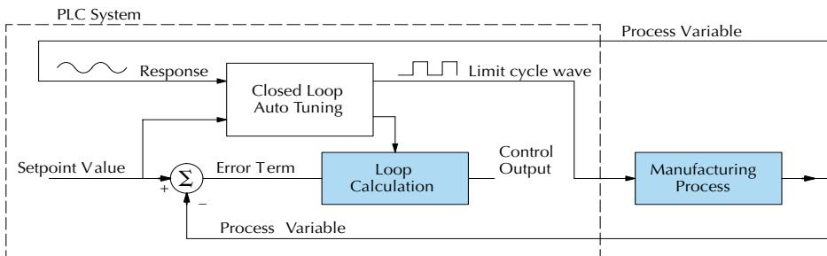
During a closed-loop auto tuning cycle, the loop controller operates as shown in the illustration below.
