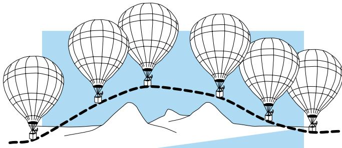
which is his control output. The large mass of air in the balloon effectively averages the effect of the burner, converting the bursts of heat into a continuous effect: slowly changing balloon temperature and ultimately the altitude, which is the process variable.
