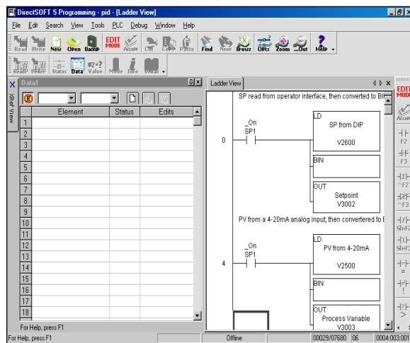
The Data View window can be used just as it is shown above for troubleshooting your PID logic, and it can be most useful when tuning the PID loop.
