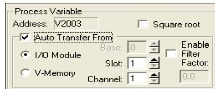
The second choice is V-Memory. When this is selected, the V-memory address from where the PV is transferred must be specified.
