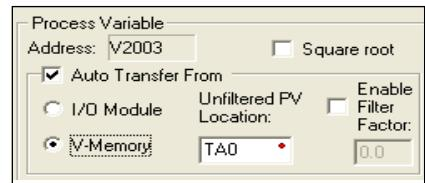
Whichever method of auto transfer is used, it is recommended to check the Enable Filter Factor (a low pass filter) and specify the coefficient.
