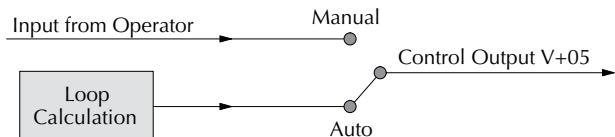
In Cascade Mode, the loop operates as it does in Automatic Mode, with one important difference. The data source for the SP changes from its normal location at V+02 to using the control output value, V+05, from another loop. So in Auto or Manual modes, the loop calculation uses the data at V+02. In Cascade Mode, the loop calculation reads the control output from another loop's parameter table, V+05.
