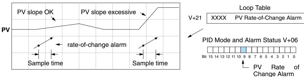
As an example, suppose the PV is the temperature for your process, and you want an alarm whenever the temperature changes faster than 15 degrees/minute. The PV counts per degree and the loop sample rate must be known. Then, suppose the PV value (in V+03 location) represents 10 counts per degree, and the loop sample rate is 2 seconds. Use the formula below to convert our engineering units to counts/sample period:
