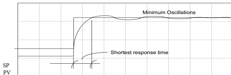
The manual method is the most common method used to tune a PID loop. Derivative gain is almost never used in a temperature control loop. This method can also be used for other control loops, but other parameters may need to be added for a stable control output.
