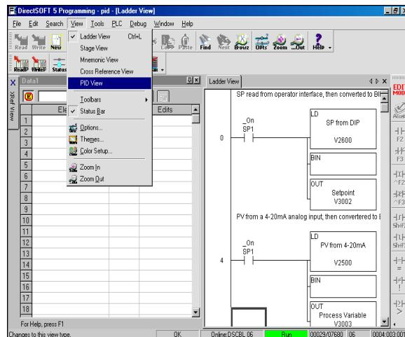
The PID View will open and appear over the Ladder View which can be brought into view by clicking on its tab. When using the Data View and the PID View together, each view can be sized for better use as shown on the facing page.
