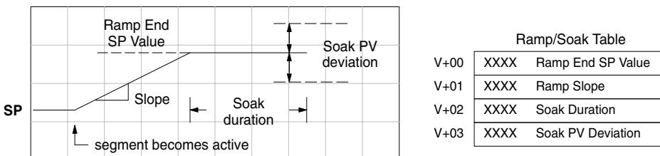
The ramp segment becomes active when the previous soak segment ends. If the ramp is the first segment, it becomes active when the ramp/soak generator is started, and automatically assumes the present SP as the starting SP.
