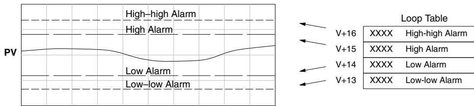
**NOTE:** The Alarm dialog can be left as it first appears, without alarm entries. The alarms can then be setup in the DirectSOFT PID View.
