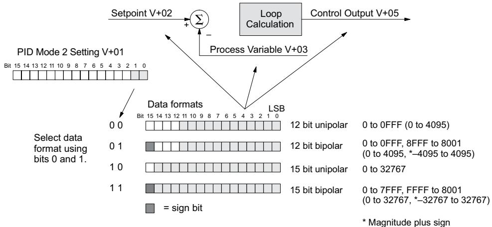
The data format determines the numerical interface between the PID loop and the PV sensor and the control output device. This selects the data format for both the SP and the PV.
