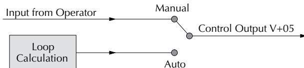
In Automatic Mode, the loop operates normally and generates new control output values. It calculates the PID equation and writes the result in location V+05 every sample period of that loop. The equivalent schematic diagram is shown below.
