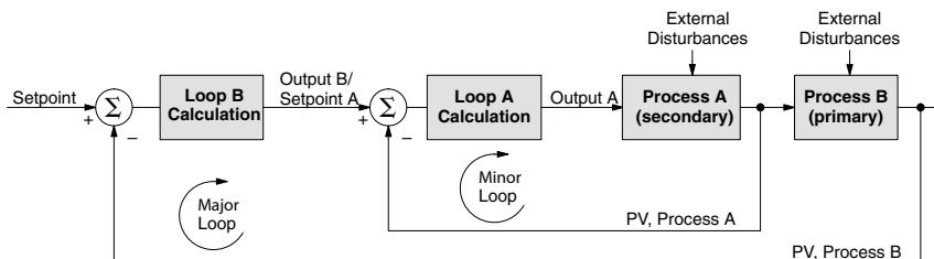
One of the benefits to cascade control can be seen by examining its response to external disturbances. Remember the minor loop is faster acting than the major loop. Therefore, if a disturbance affects process A in the minor loop, the Loop A PID calculation can correct the resulting error before the major loop sees the effect.
