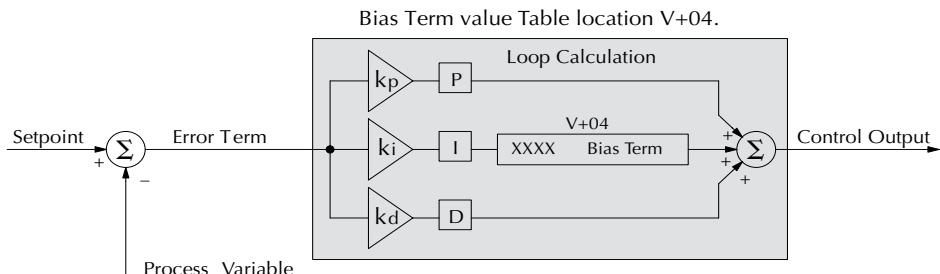
To change the bias (operating point), ladder logic only has to write the desired value to V+04. The PID loop calculation first reads the bias value from V+04 and modifies the value based on the current integrator calculation. Then it writes the result back to location V+04. This arrangement creates a sort of transparent bias term. All you have to do to implement feed forward control is write the correct value to the bias term at the right time (see the following example).
