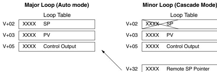
Cascade Mode, the minor loop will ignore the its local SP register (V+02), and read the major loop's control output as its SP instead.
