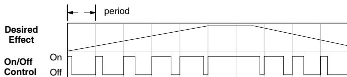
If we were to plot the on/off times of the burner in the hot-air balloon, we would probably see a very similar relationship to its effect on balloon temperature and altitude.
