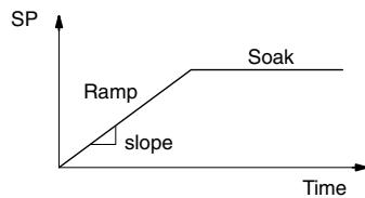
Complex SP profiles can be generated by specifying a series of ramp/soak segments. The ramp segments are specified in SP units per second time. The soak time is also programmable in minutes.
