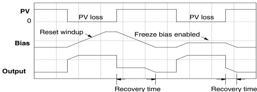
In the second PV signal loss episode in the figure, the freeze bias feature is enabled. It causes the bias value to freeze when the control output goes out of bounds. Much of the reset windup is thus avoided, and the output recovery time is much less.
