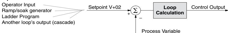
If the SP for your process rarely changes or can tolerate step changes, you probably will not need to use the ramp/soak generator. However, some processes require precisely-controlled SP value changes. The ramp/soak generator can greatly reduce the amount of programming required for these applications.
