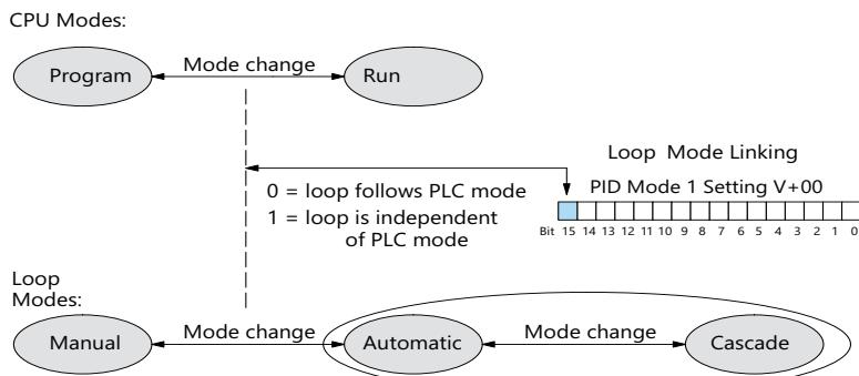
If bit 15 is set to one, then the loops will run independently of the CPU mode. It is like having two independent processors in the CPU... one is running the RLL program and the other is running the process loops.
