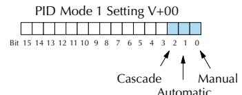
The normal state of these mode request bits is "000." To request a mode change, you must SET the corresponding bit to a "1" using a one-shot. The PID loop controller automatically resets the bits back to "000" after it reads the mode change request. Methods of requesting mode changes are:
