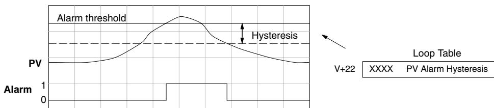
The hysteresis amount is applied after the threshold is crossed, and toward the safe zone. In this way, the alarm activates immediately above the programmed threshold value. It delays turning off until the PV value has returned through the threshold by the hysteresis amount.
