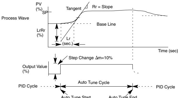
When the loop tuning observations are complete, the loop controller computes Rr (maximum slope in %/sec.) and Lr (dead time in sec). The auto tune function computes the gains according to the Zeigler-Nichols equations, shown below:
