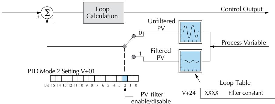
Bit 2 of PID Mode Setting 2 provides the enable/disable control for the low-pass PV filter (0=disable, 1=enable). The roll-off frequency of the single-pole low-pass filter is controlled by using register V+24 in the loop parameter table, the filter constant. The data format of the filter constant value is BCD, with an implied decimal point 00X.X, as follows:
