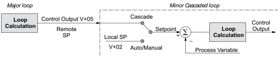
Remember that a major loop goes to Manual Mode automatically if its minor loop is taken out of Cascade Mode.
