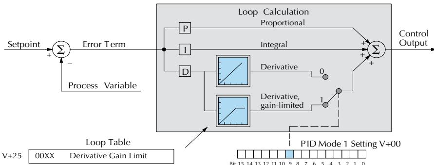
The gain limit can be particularly useful during loop tuning. Most loops can tolerate only a little derivative gain without going into uncontrolled oscillations.
