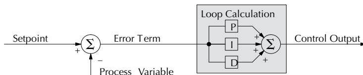
The P, I and D gains are 4-digit BCD numbers with values from 0000 to 9999. They contain an implied decimal point in the middle, so the values are actually 00.00 to 99.99. Some gain values have units – Proportional gain has no unit, Integral gain may be selected in seconds or in minutes, and Derivative gain is in seconds.
