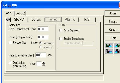
Recall the position and velocity forms of the PID loop equations which were introduced earlier. The equations basically show the three components of the PID calculation: Proportional Gain (P), Integral Gain (I) and Derivative Gain (D). The following diagram shows a form of the PID calculation in which the control output is the sum of the proportional gain, integral gain and derivative gain. With each calculation of the loop, each term receives the same error signal value.
