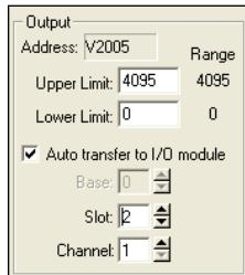
You should also select the analog output for the control output to be transferred to. This is done in the PID setup Output dialog shown here. The block of information in this dialog is grayed-out until the box next to Auto transfer to I/O module is checked. Once checked, enter the slot number where the output module is residing and then enter the analog output channel number.
